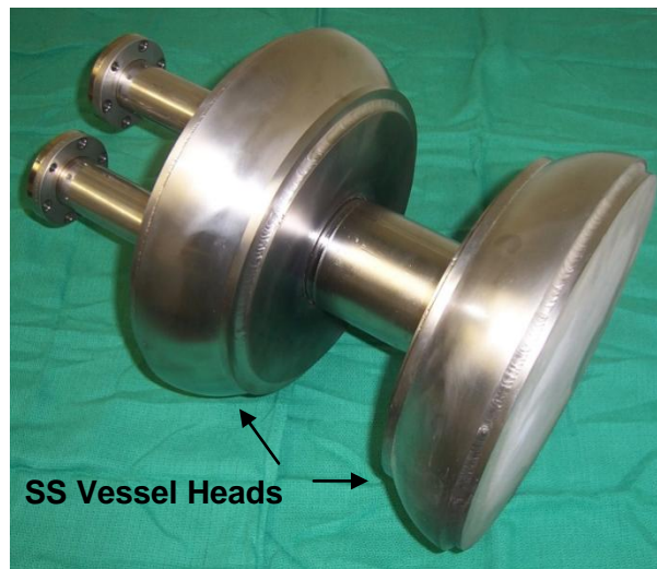
Fig. 6 Specially designed pressure test fixture for SS vessel heads.
