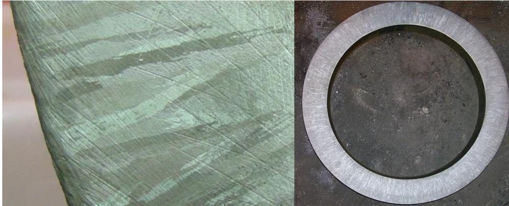
**Figure 2:** Casting cross-section macro-etched with Hydrogen Peroxide and Muriatic Acid, displaying direction solidification and grain growth from the outer diameter to the inner diameter.
