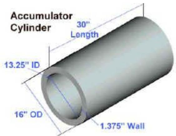
**Figure 4:** On-Ship Hydraulic Accumulators - Energy storage basin in which hydraulic fluids are held under pressure by a peripheral source.
