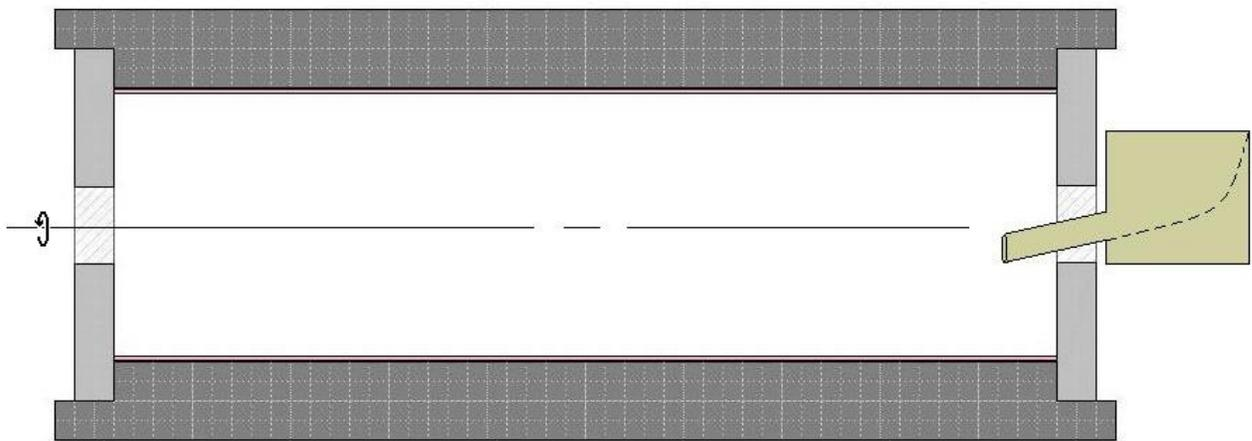
**Figure 1:** Cross-Section of a Horizontal Die with a Line Designating its Axis of Rotation.
